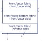
With front/outer sides facing each other, piece together the front/outer fabric and bottom fabric.
