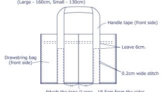
Attach the tape (Large - 18.5cm from the sides, Small - 13.5cm from the sides)
