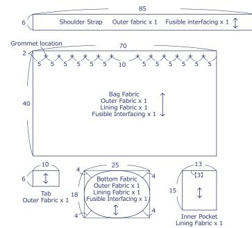
\*Adhere fusible interfacing on the back of the shoulder strap. outer bag fabric and outer bottom fabric.
