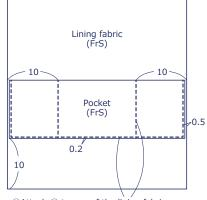
3 Attach 2 to one of the lining fabrics and sew the partition.
