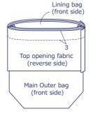
2 With front sides facing each other, sew together the outer bag and top opening fabric.
