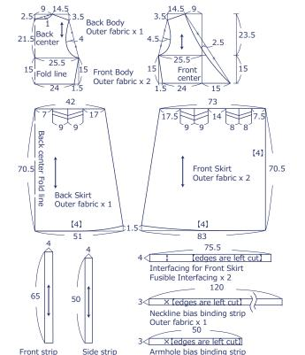
\* Adhere fusible interfacing on the front edge of the seam of front skirt.
