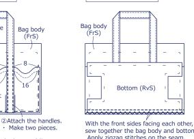
sew together the bag body and bottom. Apply zigzag stitches on the seam.
