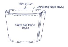
5. Turn it inside out and apply stitches around the top opening
