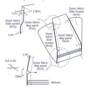
4. With the front sides facing each other, layer the outer fabric and lining fabric and sew together at the top opening
